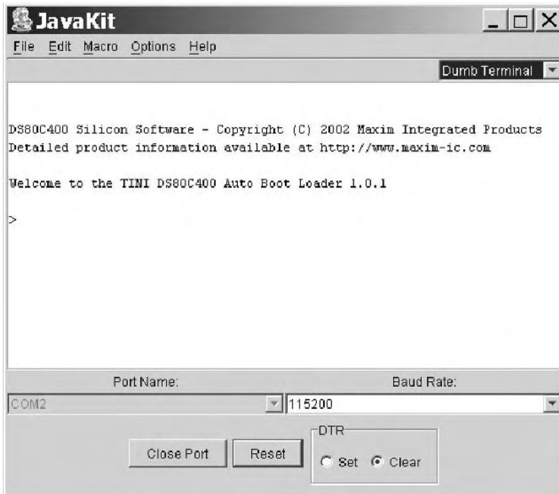
Figure 3-7: The JavaKit utility enables you to start the TINI’s JVM and run the slush command shell.
