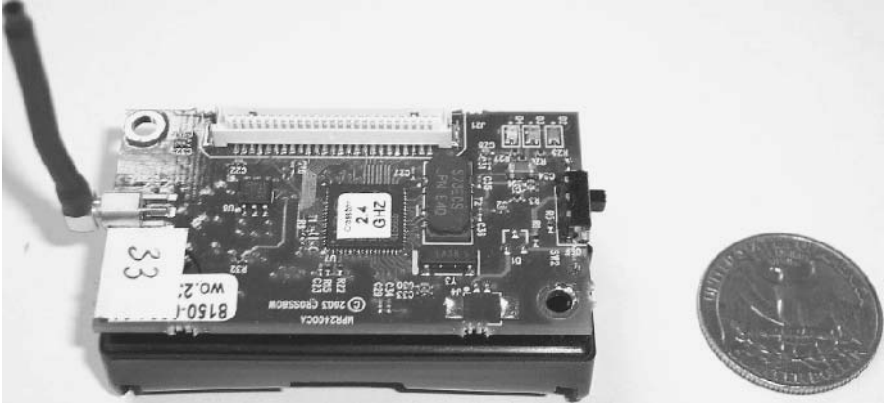
Figure 1.1 A Berkeley mote (MICAz MPR2400 series)
