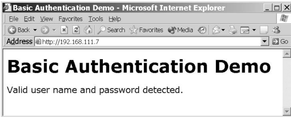
Figure 10-2: On receiving a valid user name and password, the application returns the requested Web page.
