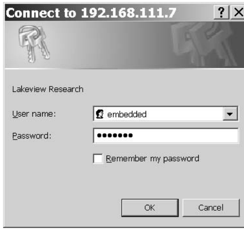
Figure 10-1: On receiving a request for Basic Authentication, browsers display a window like this to enable users to enter a user name and password.
